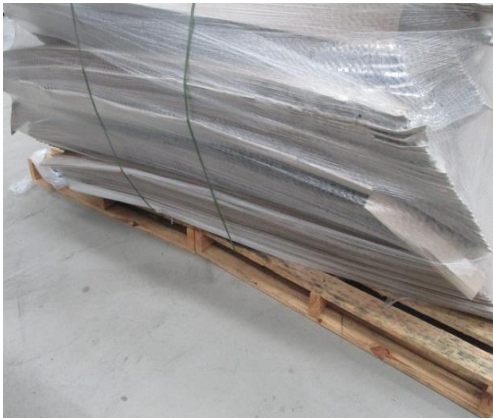
Example: poor use of plastic strapping.
