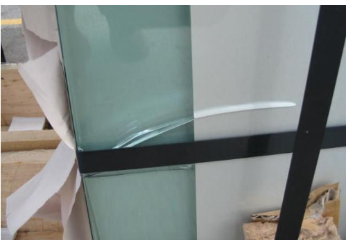
Example: poor use of metal strapping
