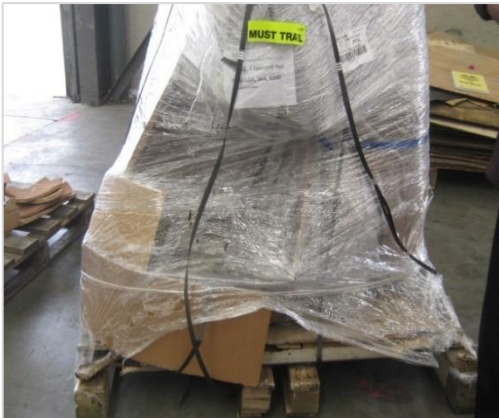
Example: poorly strapped goods, straps have loosened in transit.
